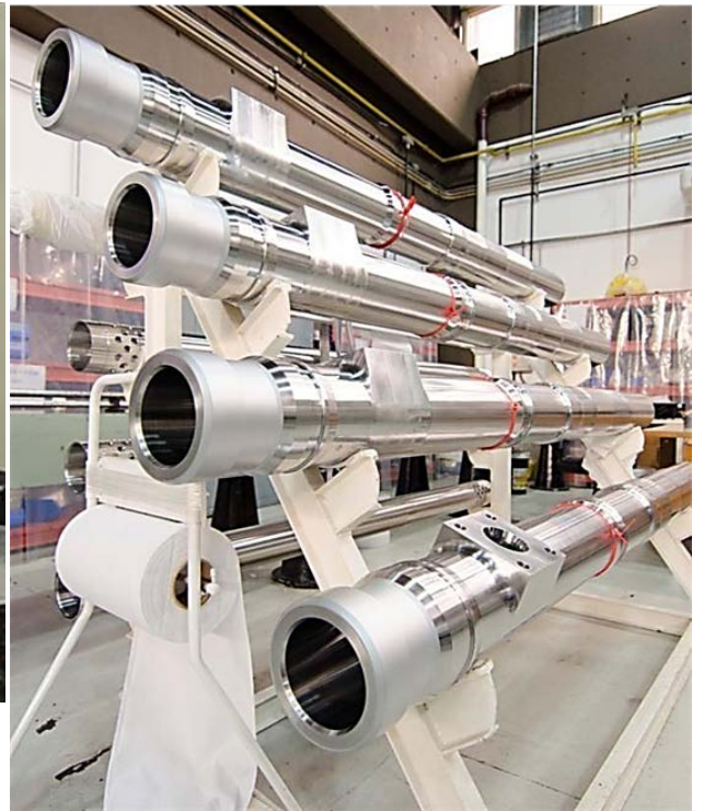
Manufacturing and assembly of two Moderator Heat Exchangers - Embalse CANDU®6 NPP Refurbishment
