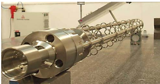
R.O.B.I.N. "basket" device for testing hi-tech optical fibers at high radiation environments. Belgium BR2 M.T.Reactor - SCK·CEN
