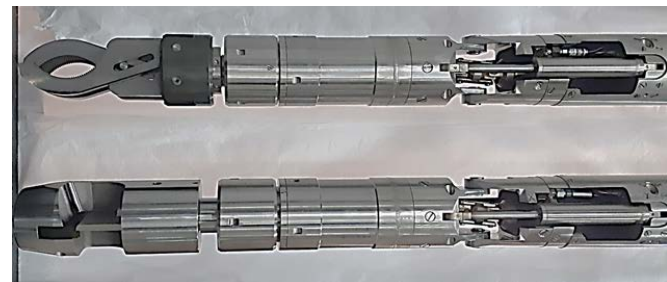
Remote Controlled Articulated Tools for performing maintenances inside Atucha I & II reactors.
