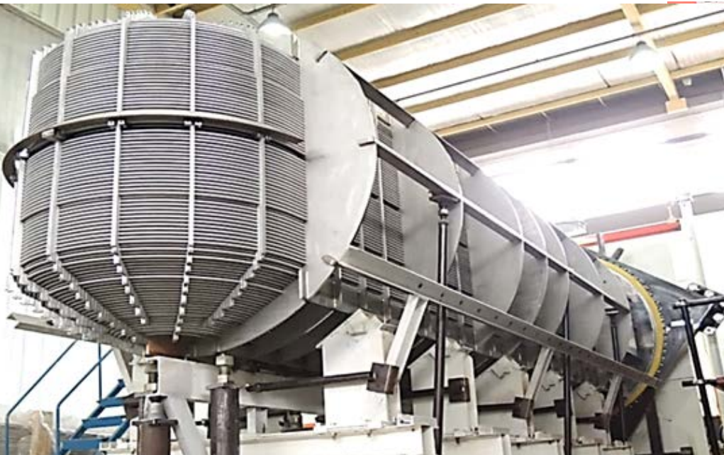
Manufacturing and assembly of two Moderator Heat Exchangers - Embalse CANDU®6 NPP Refurbishment
